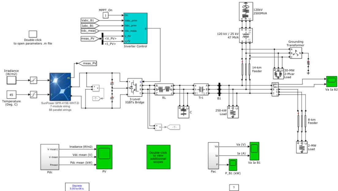
Fig 4: PV designed model
