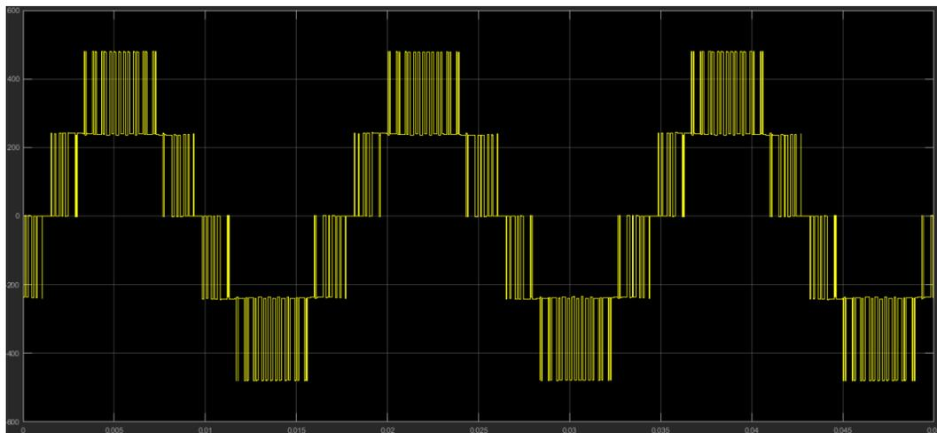
(a) Unfiltered Inverter output voltage
