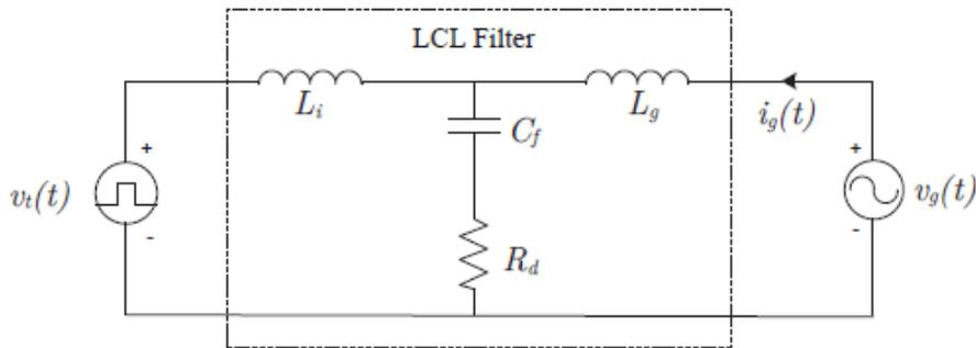
Fig.2: L-C-L filter and components [2]
